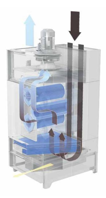
The air entry section, which connects the piping to the filter, consists in a large area which serves as a calming chamber. Inside this area a pre-blasting system "Twist" (optional) can be provided which further facilitates the aggregation of the finer particles by means of a forced, centrifugal effect. Subsequently, the air passes through two separate and reusable filtration stages, a PVC drop separator and a metallic G3 filter.
