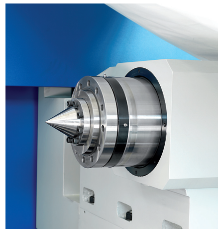
TAILSTOCK. The tailstock is clamped to the bed using disc type springs and hydraulic unclamping. Oversized bearings, maximum quill adjustment accuracy, axial dilatation compensation and strength pressure regulator.
