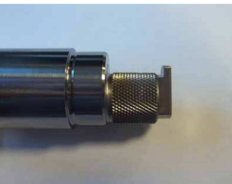
The component part is an eccentric turned part made of high-tensile stainless steel.
