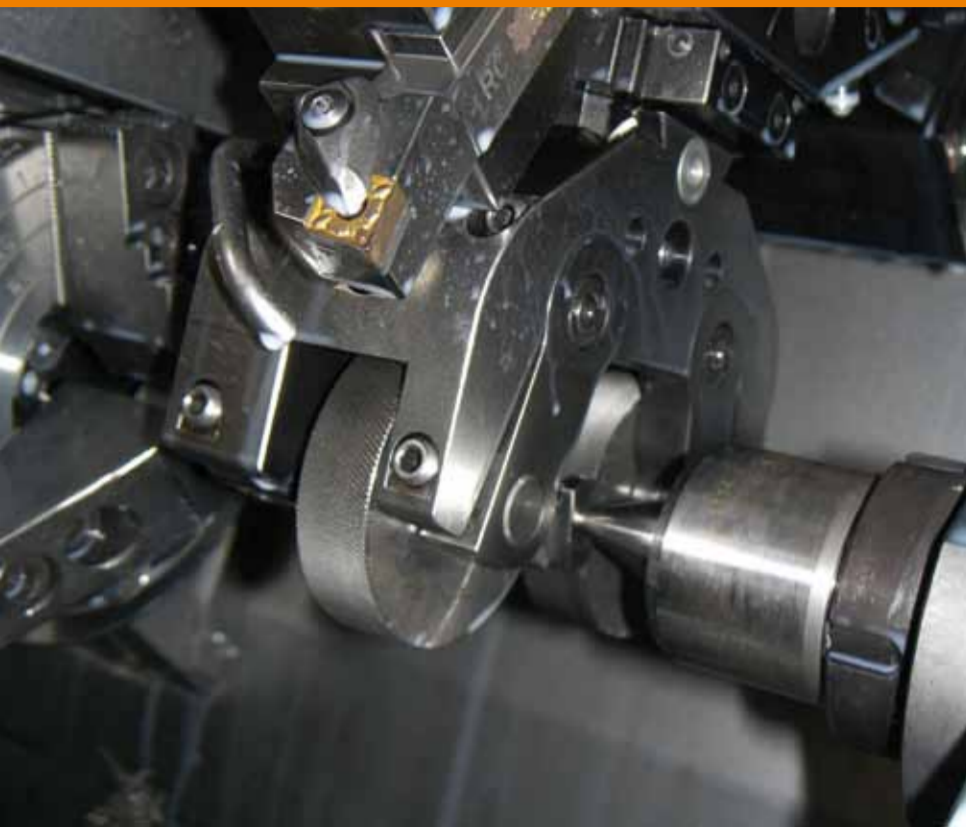
► Fig.: HN-Metallbearbeitung also uses axially driven tools from WAGNER®, which are used for milling component parts.
