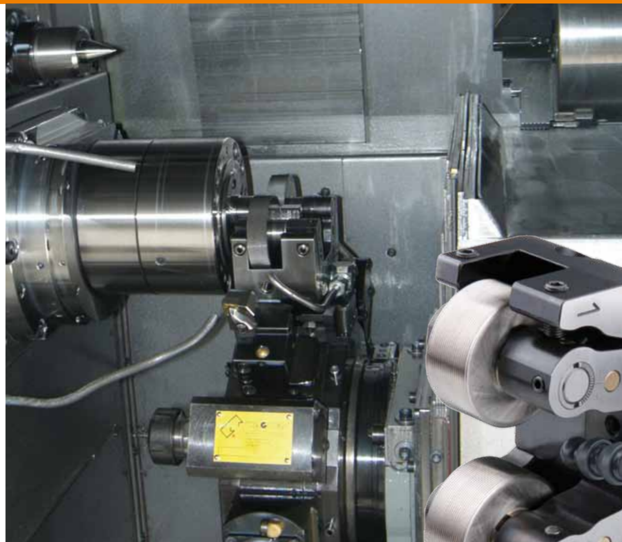
► Fig.: HN-Metallbearbeitung also uses axially driven tools from WAGNER®, which are used for milling component parts.
