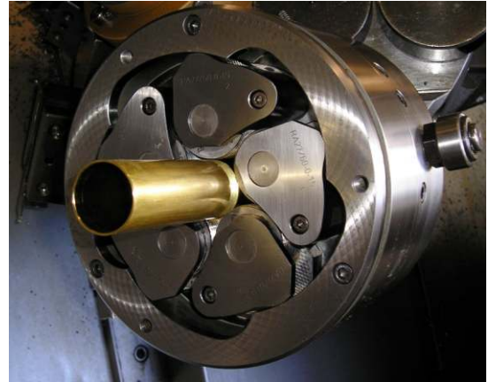
Rolling on pipes with WAGNER® RS 60-5
